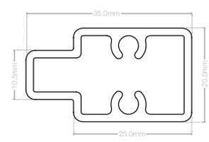
Mechanical joint / reinforcement for midrail
