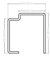
Reinforcement For door sash
